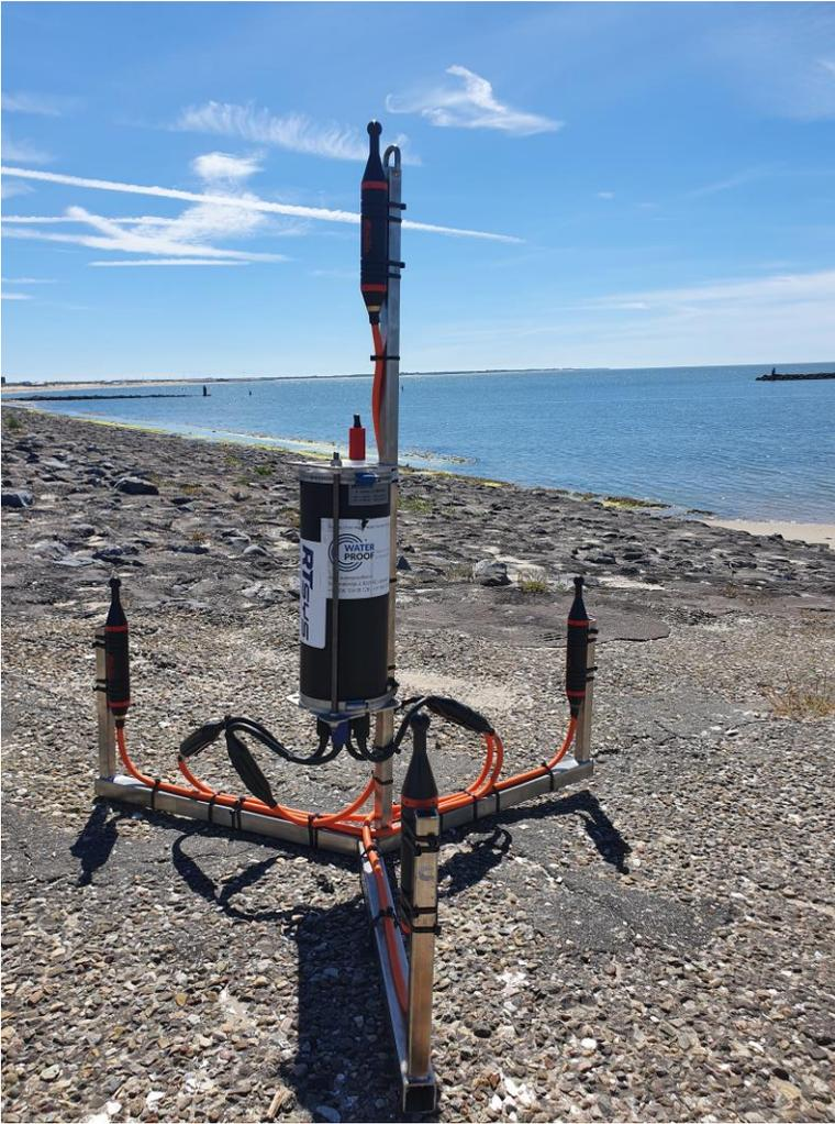
*Figure 0-2 HPTS test station, with four hydrophones for triangulation.*
