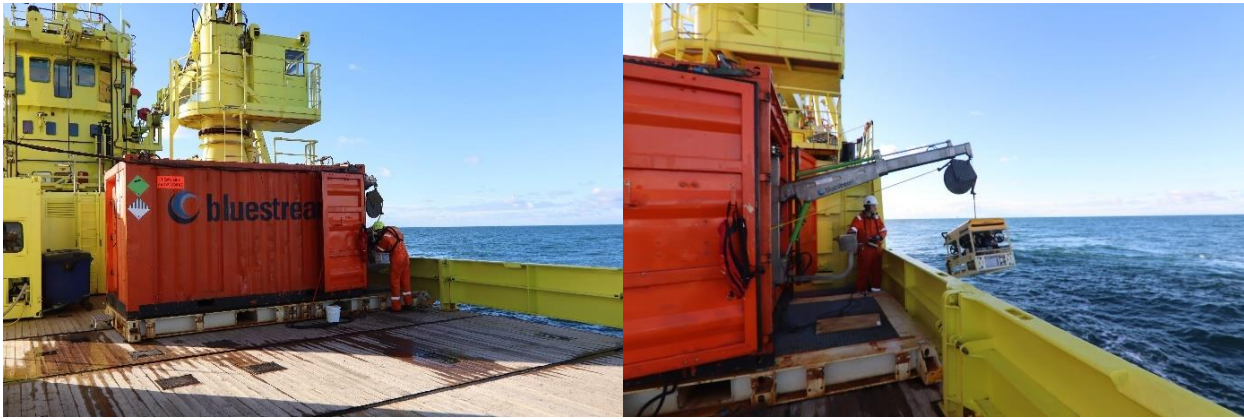
Figure 3.2 Left: The ROV container on deck, right: deployment of the ROV from the container (photos by Joop Coolen, WMR).
