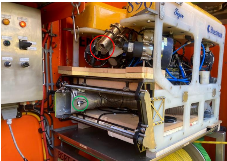
Figure 3.3 Positions of the cameras with red: overview camera on the ROV and green: close-up camera near the scraper (photo by Joop Coolen, WMR).
