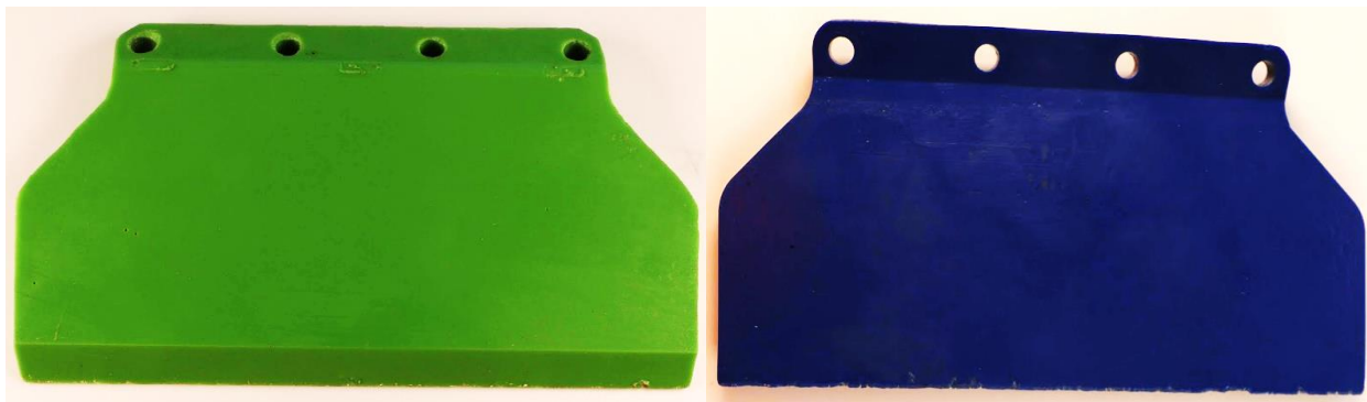
Figure 4.4 Green and blue scraper with damage (bottom sides in photos) after scraping 4 samples each.
