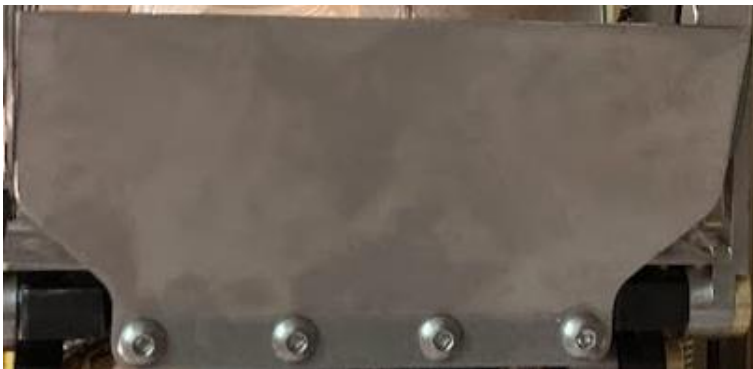
Figure 3.5 Metal scraper used in the MGST. See results section for plastic scrapers.
