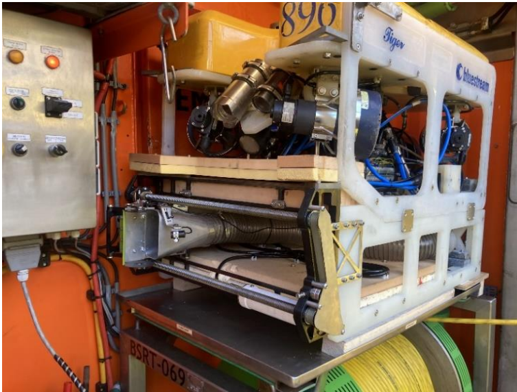
Figure 1.1. The MGST mounted under the Saab SeaEye Tiger ROV, ready to be deployed for the sampling test (photo by Joop Coolen, WMR).
