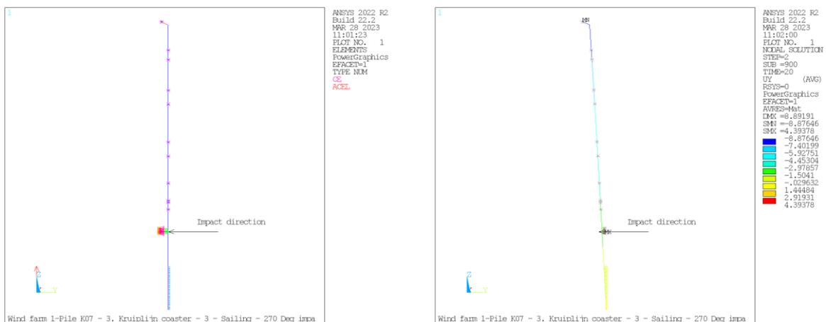
Figure 9.4: Impact directly below the nacelle of the turbine impact in the negative Y-direction.
