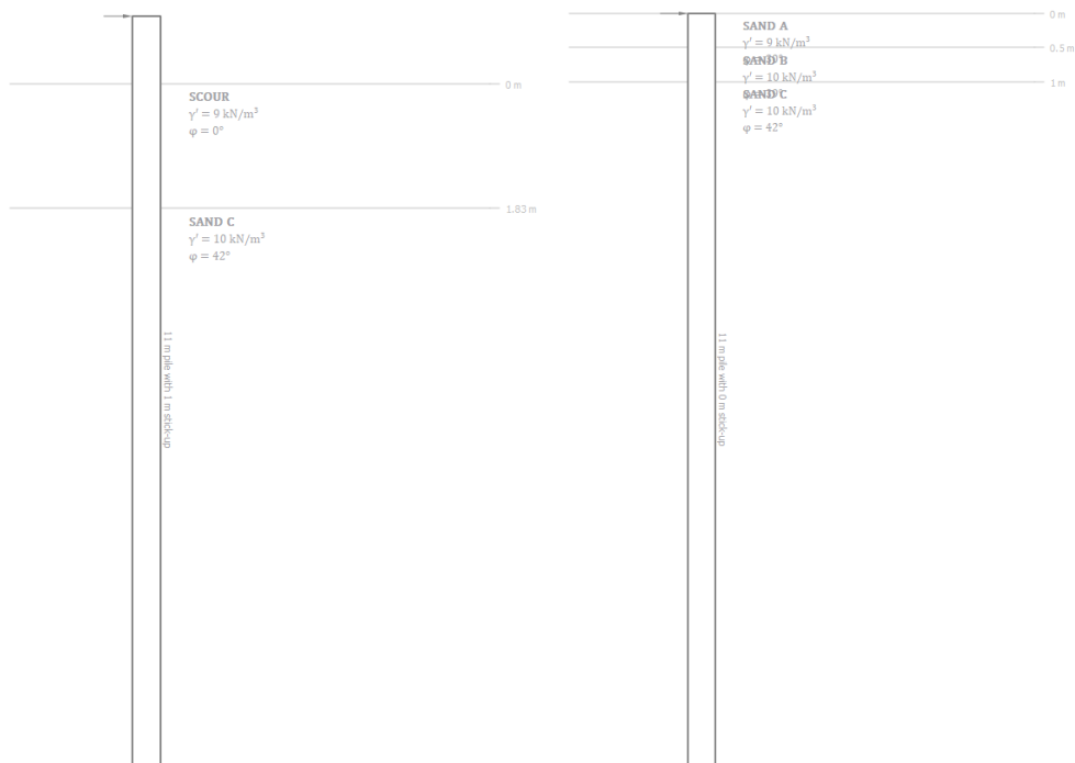
Figure 5: Pile model in PyPile, with and without scour. With scour the stick out (global scour) is 1.0m.
