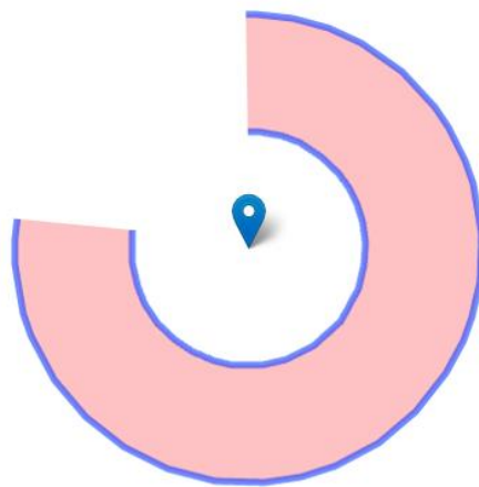
Figure 2.1 Donut-shaped area which was used to calculate the MTR from the horizontal radar data. The blue marker shows the radar position. The white triangle represents the blanking area of the radar to avoid radiation from the turbine on which the radar is installed.
