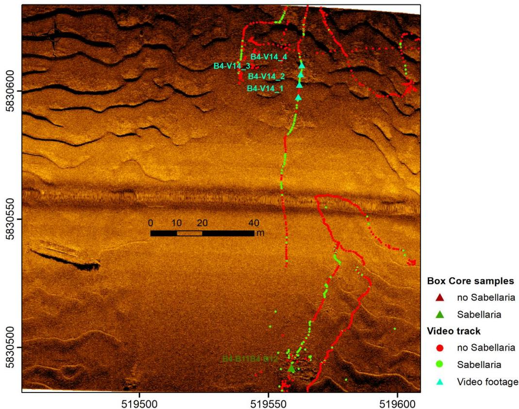
Figure 4.10: SSS image showing ship wreck and indicative patterns for elevated *Sabellaria spinulosa*. Light blue dots mark positions of video footage shown in Figure 4.12. Residue from boxcore B4-V11 (denoted in dark green) is shown in Figure 4.13. Boxcore B4-V12 was taken at the same position.
