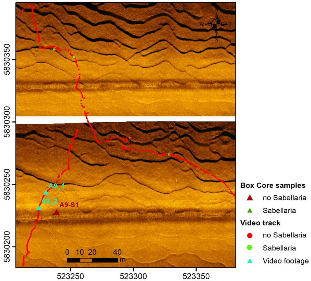
Figure 4.7: Subset of Area A showing SSS backscatter. Boxcore locations and video tracks are classified to show the absence and presence of *Sabellaria*.
