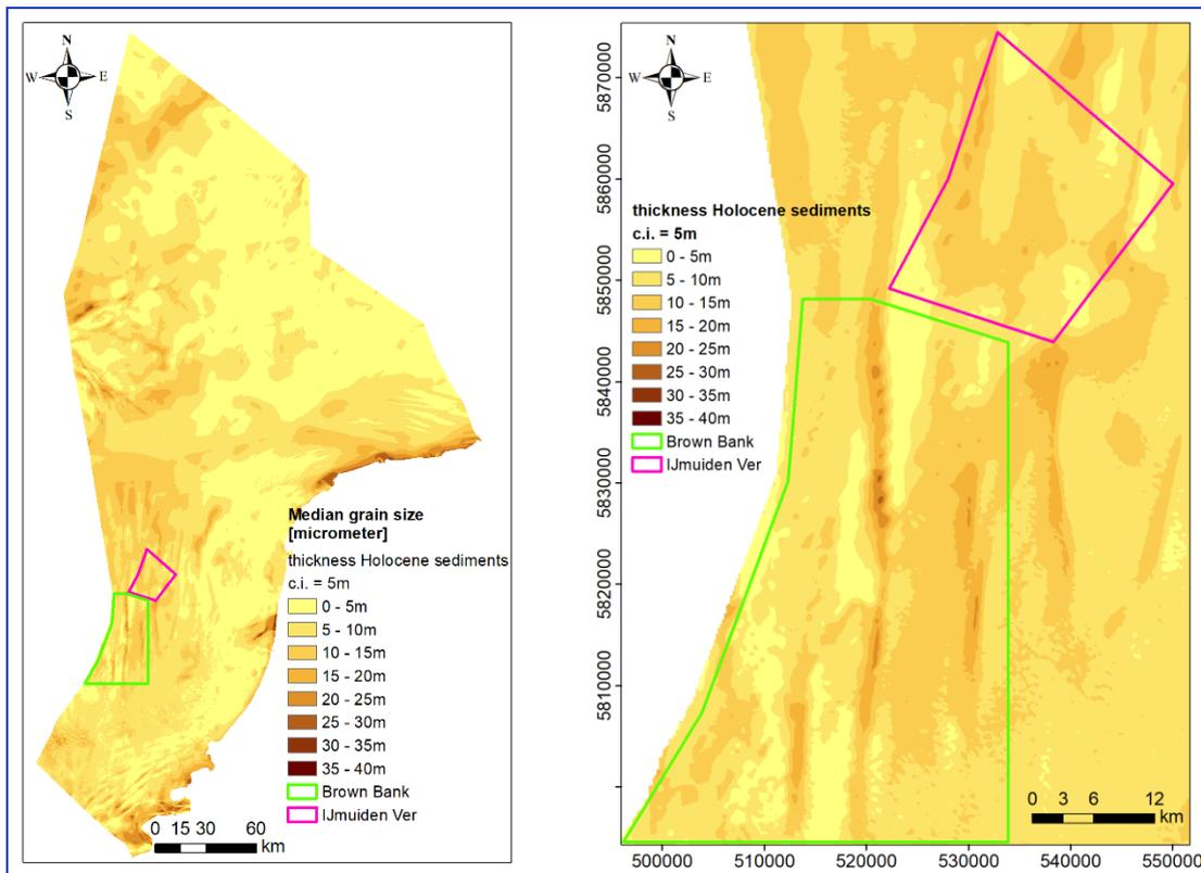
Figure 2.9: Thickness of Holocene cover of the NCS (left) and zoom-in sections Brown Bank and IJVER (right).
