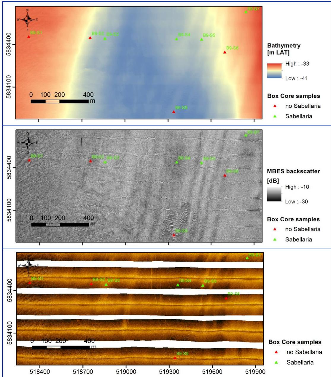
Figure 4.14: Northern part of Area B with distribution of flat/buried *Sabellaria* structures. (Top) MBES bathymetry, (middle) MBES backscatter and (bottom) SSS backscatter.
