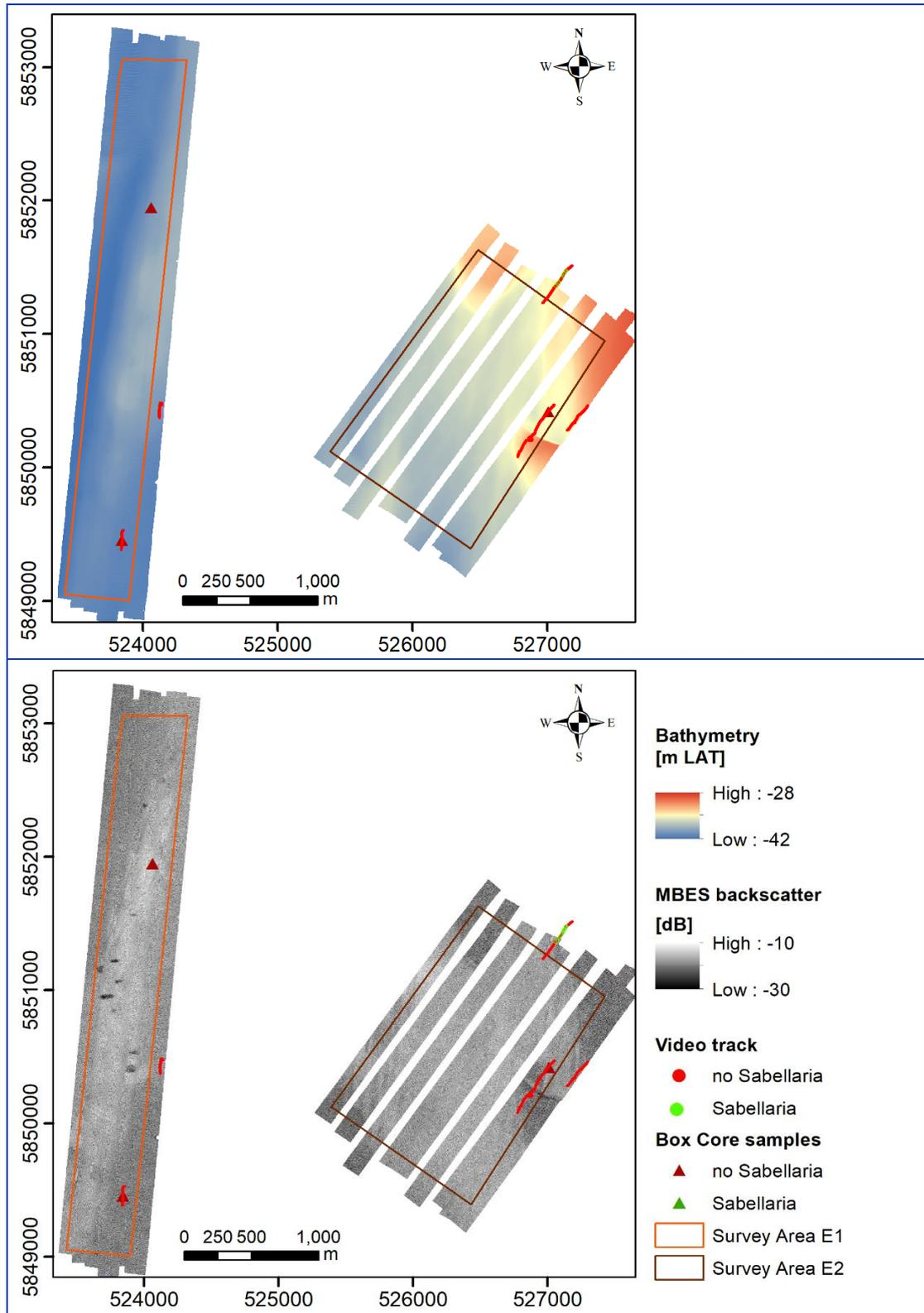
Figure 4.16: Mapped Area E1 (left) and E2 (right) with (top) MBES bathymetry and (bottom) MBES backscatter. In both maps, boxcore locations as well as video tracks are classified to show the presence and absence of *Sabellaria*.
