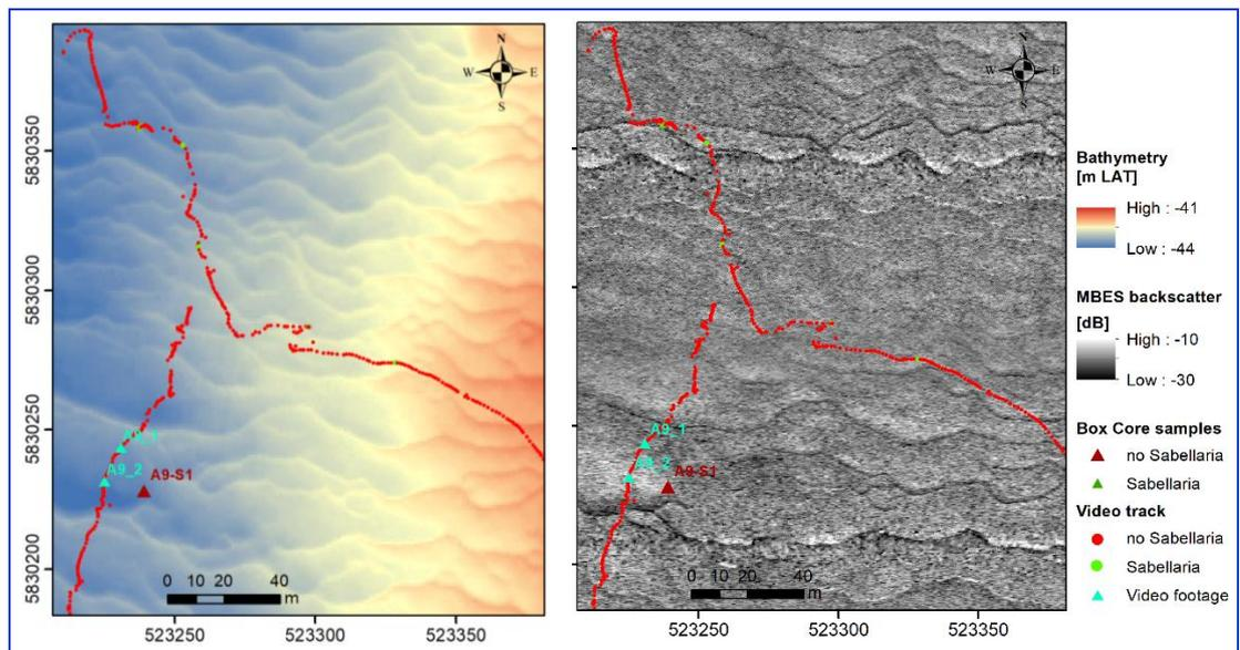
Figure 4.6: Subset of Area A showing (left) MBES bathymetry and (right) MBES backscatter. In both maps, boxcore locations as well as video tracks are classified to show the absence and presence of *Sabellaria*.
