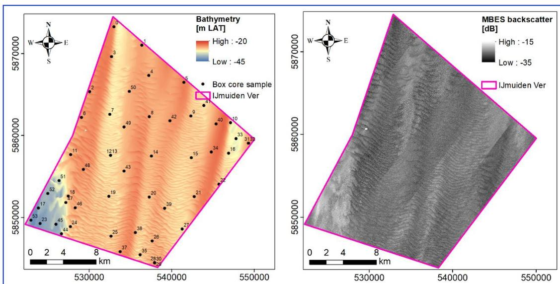
Figure 2.2: IJVER MBES bathymetry with sample locations (black dots) (left) and MBES backscatter (right).
