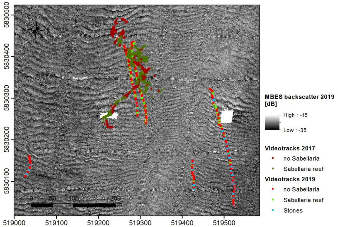
Figure 2.5: Example of combination of video recordings and high resolution MBES backscatter acquired with a Kongsberg EM302 at 30 kHz in DISCLOSE project in 2019. Green dots show presence of *Sabellaria* reefs and red dots show absence. In 2019 an additional class of stones (blue dots) was added. The white rectangular spots in the middle of the figure are data gaps and shouldn't be mistaken with the max backscatter value.
