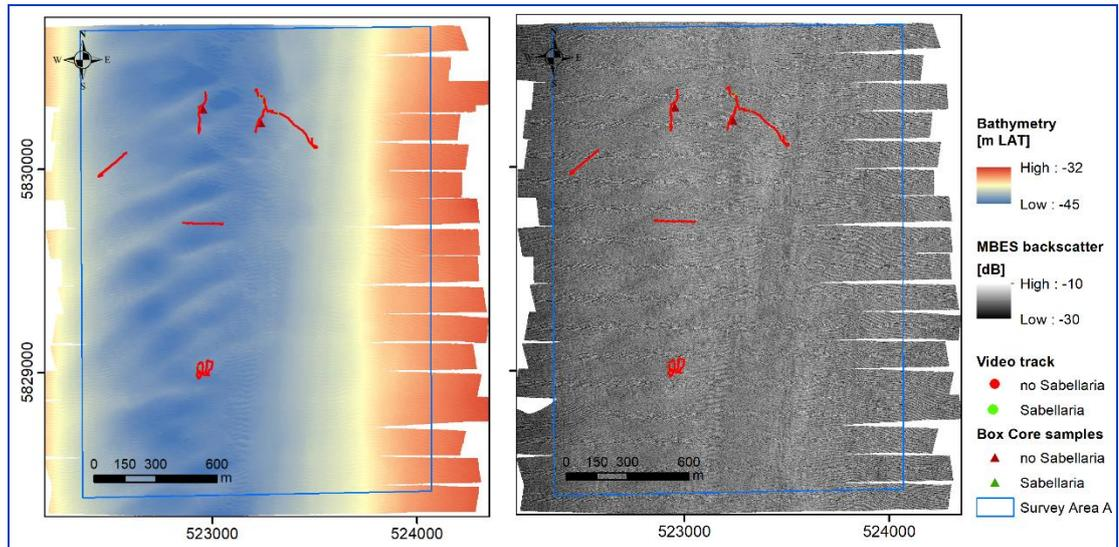
Figure 4.5: Mapped Area A with (left) MBES bathymetry and (right) MBES backscatter. In both maps, box-core locations as well as video tracks are classified to show the absence and presence of *Sabellaria*.
