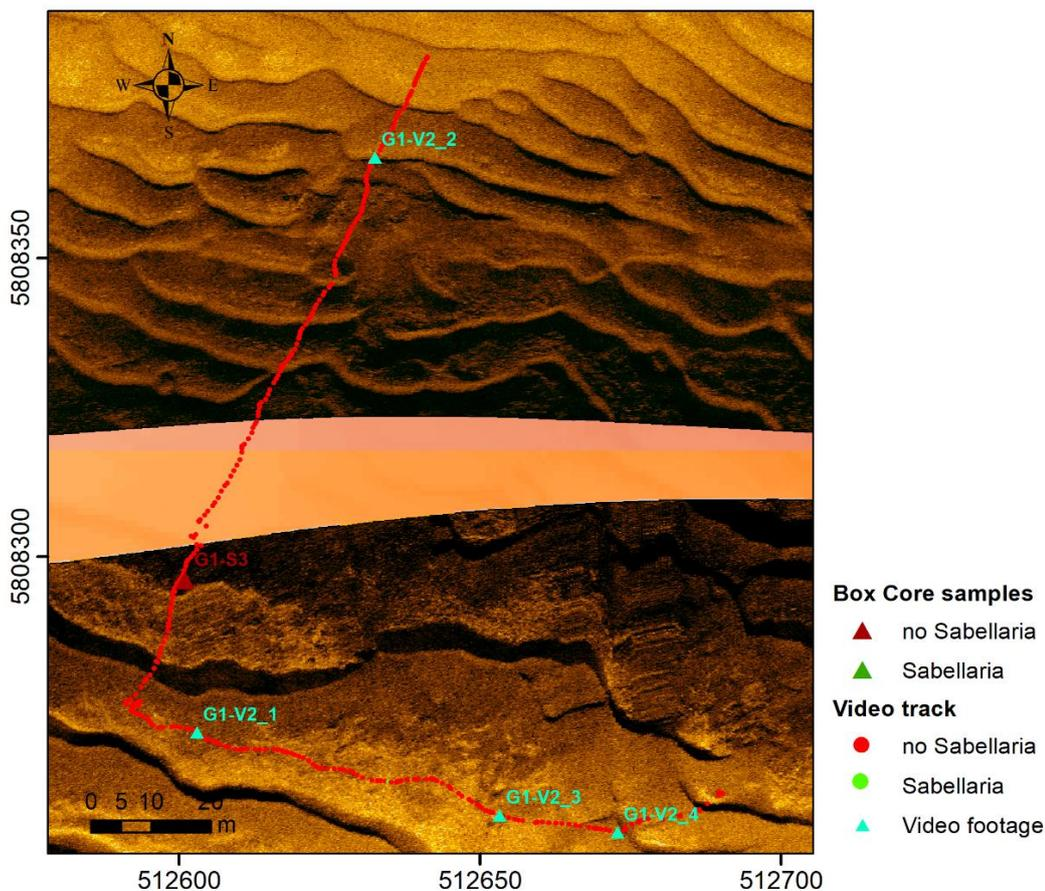
Figure 4.28: Subsection of Area G showing SSS backscatter. Boxcore locations and video tracks are classified to show the presence and absence of *Sabellaria*.
