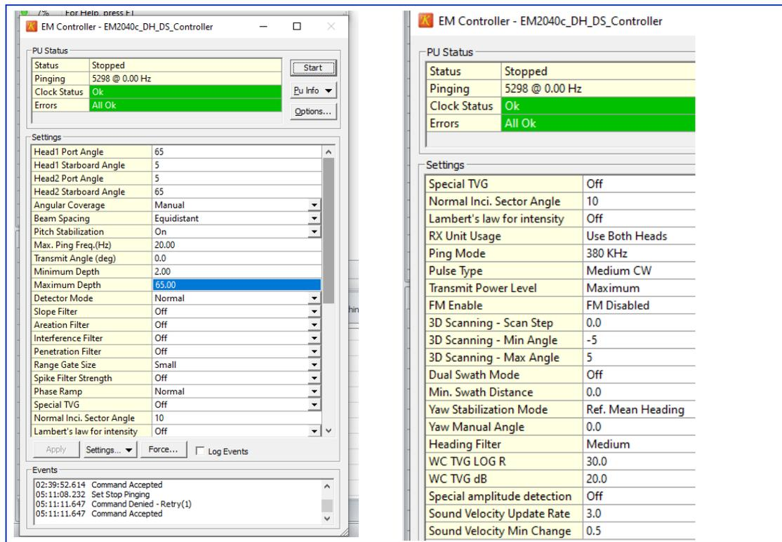
Figure A.1: The MBES settings and filters used during the trial.
