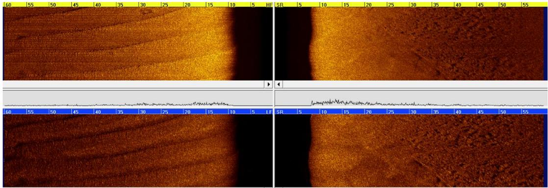
Figure 2.15: SSS waterfall display showing the typical *Sabellaria spinulosa* pattern (right side). The image is from the same location as the outlined section in Figure 2.14.
