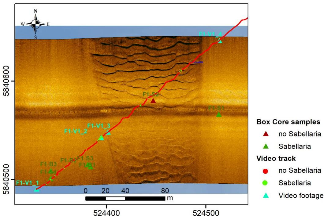
Figure 4.24: Subsection of Area F showing SSS backscatter, highlighting the extent of a megaripple field. Boxcore locations and video tracks are classified to show the presence and absence of *Sabellaria*.
