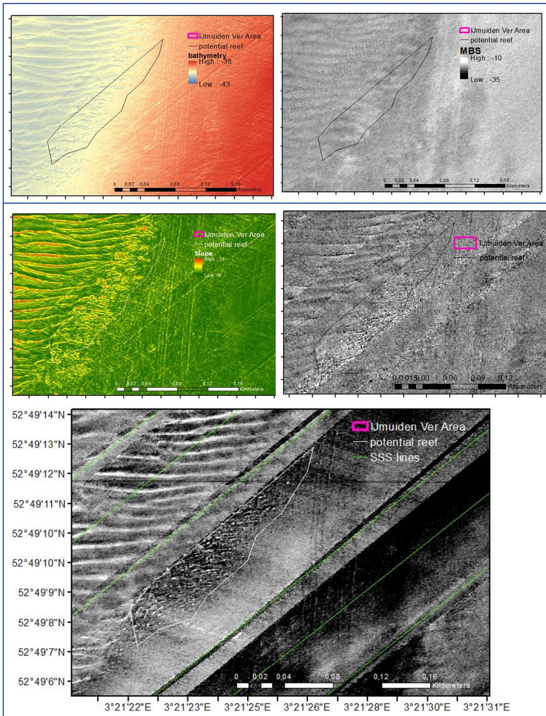
Figure 2.14: Selected area in IJVER (SW-NE outline) that could potentially contain *Sabellaria* reefs. This example region is located in survey area E. (Top left) MBES bathymetry, (Top right) MBES backscatter mosaic, (Middle left) MBES bathymetry slope, (Middle right) SSS high-frequency backscatter mosaic and (bottom) SSS low-frequency backscatter mosaic.
