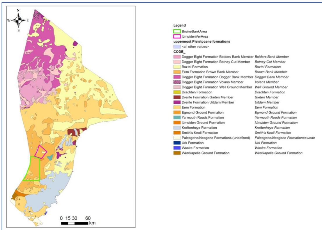
Figure 2.10: Top unit of Pleistocene subsurface sequence of the NCS (left) and zoomed-in sections Brown Bank and IJVER (right).
