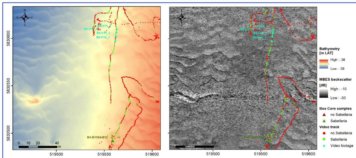
Figure 4.11: Same subset of Area B as in Figure 10, showing (left) MBES bathymetry and (right) MBES backscatter. In both maps, boxcore locations as well as video tracks are classified to show the presence and absence of *Sabellaria*.
