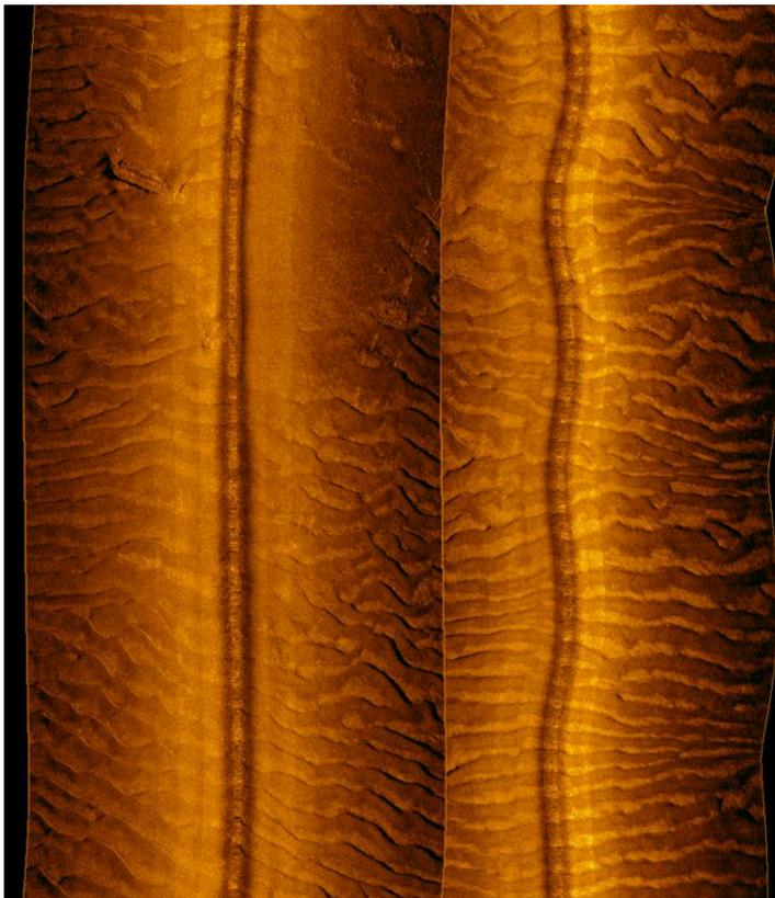
**Figure 4.4:** SSS images obtained from setting test showing *Sabellaria* findings around ship wreck. The track lines are orientated N-S and range of 75 m was used. The left track line has a flying height of 6.6 m and survey speed of 6.7 knots and the right track line a flying height of 6.6 m and a survey speed of 5.2 knots.
