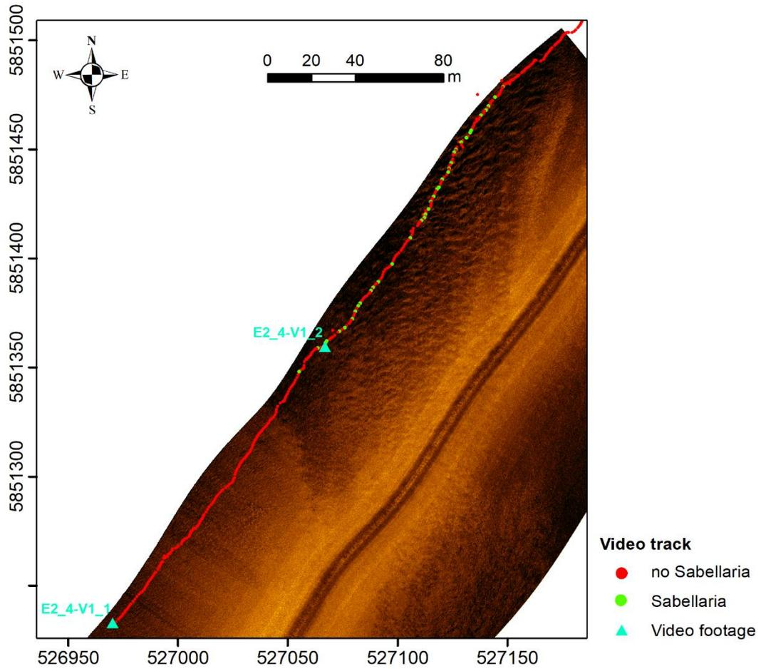
Figure 4.18: Subsection of Area E2 showing SSS backscatter. Boxcore locations and video tracks are classified to show the presence and absence of *Sabellaria*. In the SSS image, *Sabellaria* patches are represented by a blotchy pattern that is quite extensive.
