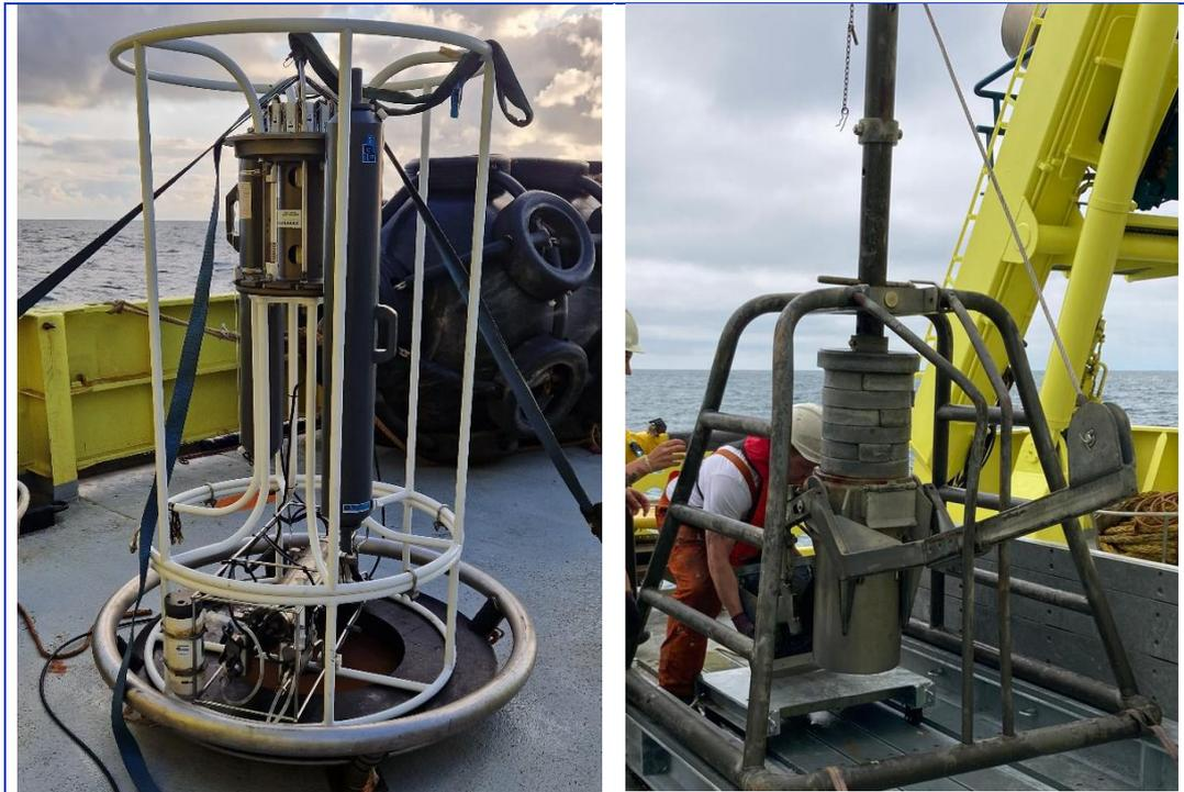
Figure 3.2: CTD-probe (left) and boxcorer (right).
