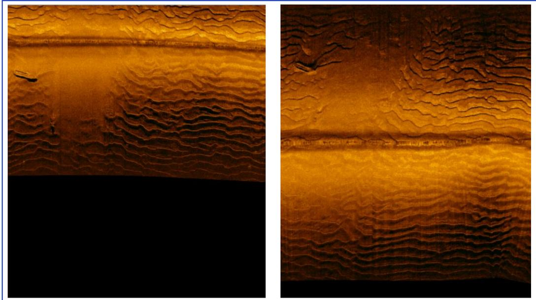
**Figure 4.3:** SSS images obtained from setting test showing *Sabellaria* findings around ship wreck. The constant parameter in these images is a range of 150 m. (Left) flying height 7.5m. (Right) flying height 14 m.
