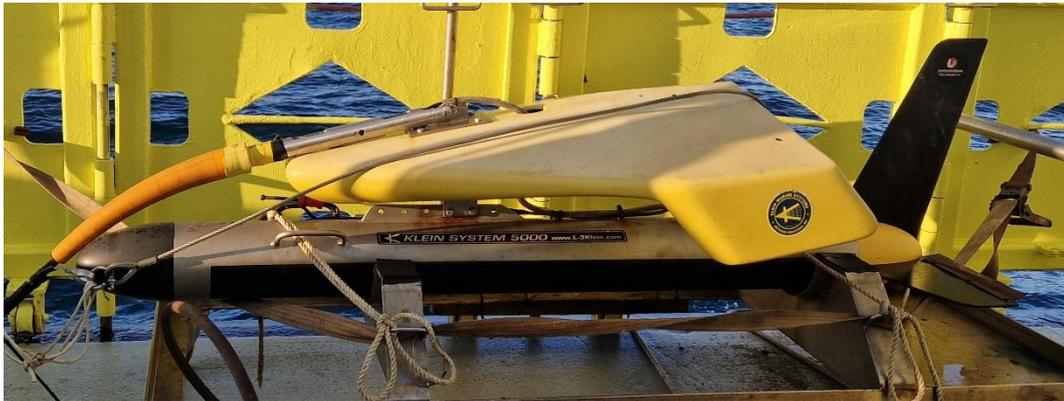
**Figure 3.1:** Klein 5000 SSS, operating at 455 kHz, and attached wing.
