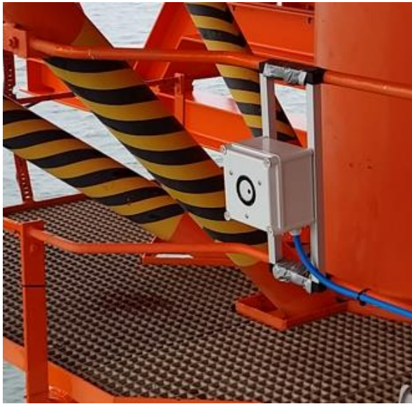
Figure 2-2. Ultrasound microphone at Lichteiland Goeree.
