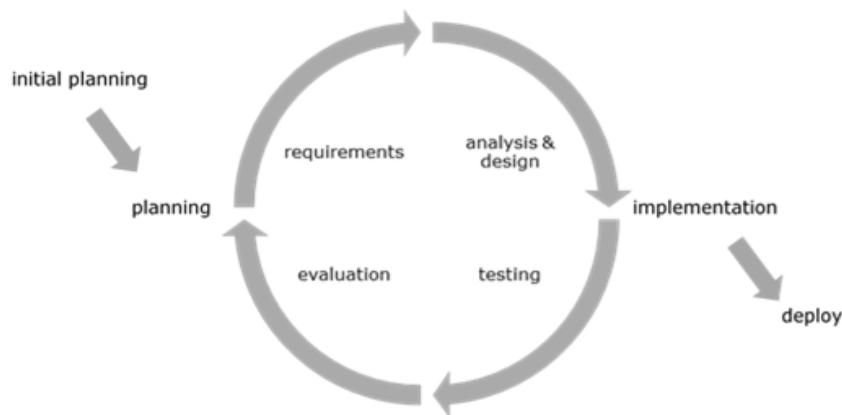
Figure 12. Schematic depiction of an agile development process, each cycle is called a 'sprint' and each sprint results in an implemented 'minimum viable product'.
