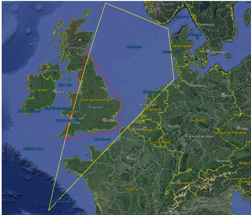
Figure 2.2. Geofences covering the North Sea and English Channel within which GPS fix interval set to 10 minutes and data download to 30 minutes (yellow) and covering the UK within which GPS fix interval set to a base rate of initially every 30 minutes and download every eight hours and later to a two-hour fix rate and a 40 hour download rate (red). Outside the geofences the base rate is used.
