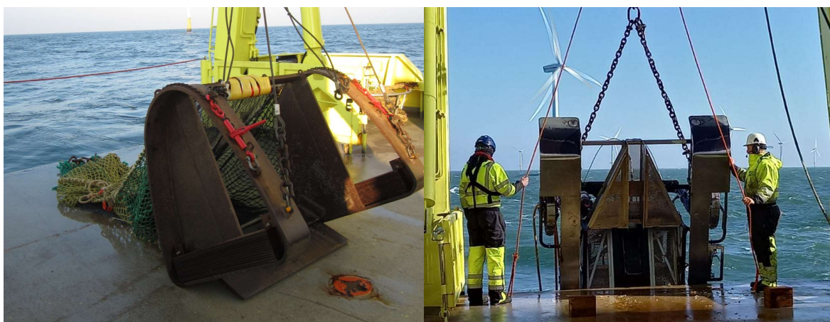
Figure 3-2: Benthic dredges used in T0 – T10 (left) and T15 (right, Triple-D)
