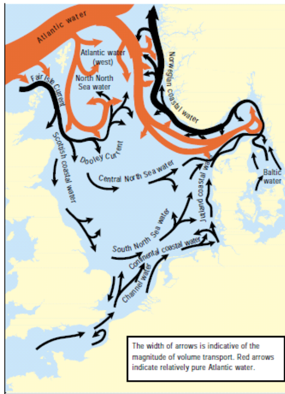
Figure 1.4 Schematic presentation of the residual water transport pattern in the North Sea (OSPAR)
