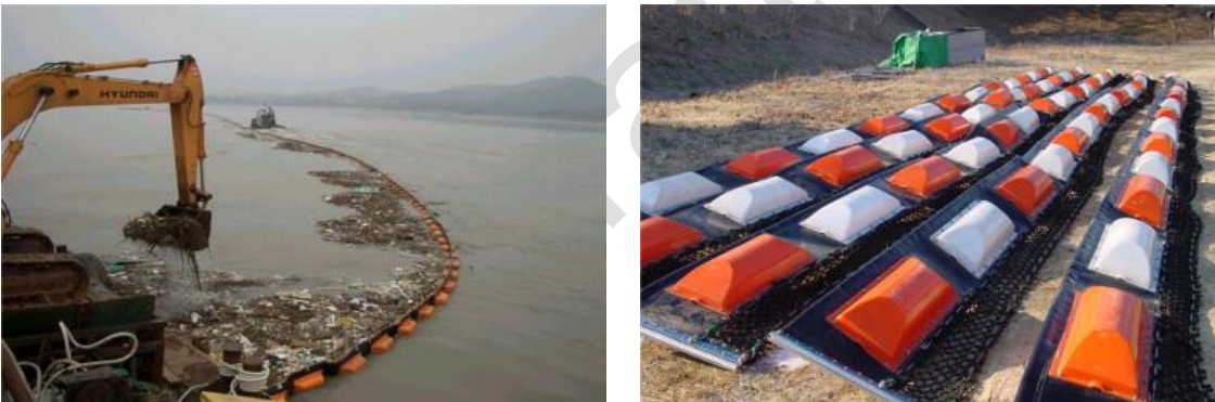
Figure 3.5 Example of a developed containment boom for floating debris in rivers (Hwang en Ko, 2007)
