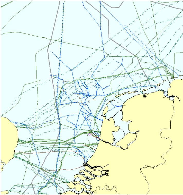
Figure 3.6 Map showing the network of cables (green) and pipelines (blue) in the North Sea (noordzeeloket.nl).
