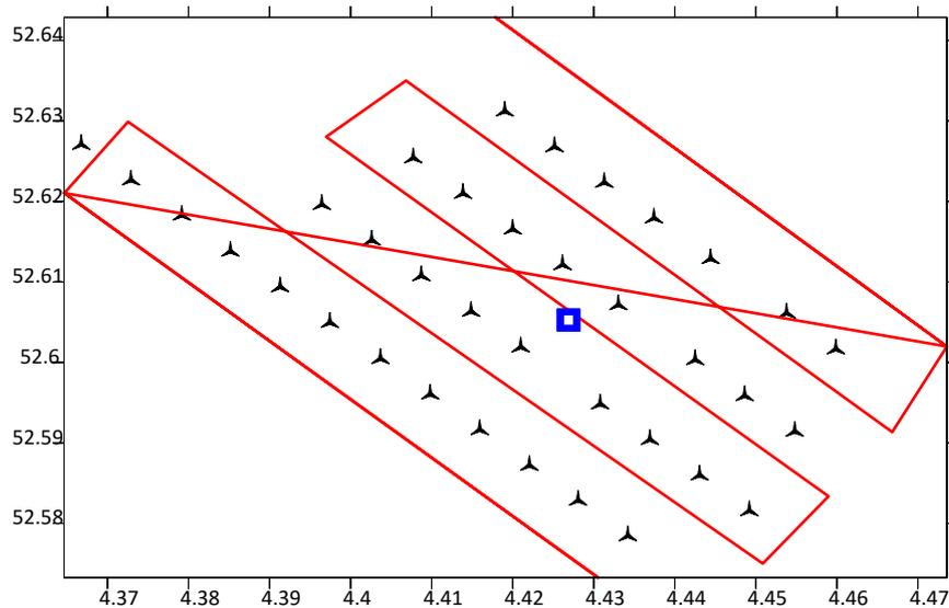
**Figure 5.11** Example of possible repetitive transect sailing (red line) of a Sailable drone in a wind farm (Egmond aan Zee). The blue rectangle is the location of the Wbat which simultaneously collects acoustic data at one spot.
