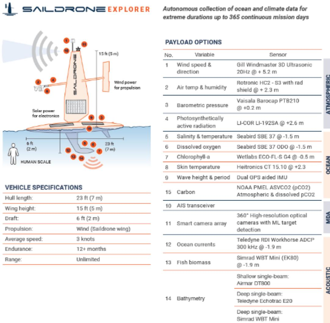
**Figure 5.12** This diagram shows the Sailable drone Standard Sensor Suite. Please note that the ADCP (sensor 12) and the Echo Sounder (sensor 13) cannot be placed on the same USV as they cannot run simultaneously. In the MONS setup, the Sailable drone carries a WBT Simrad Mini (EK80).
