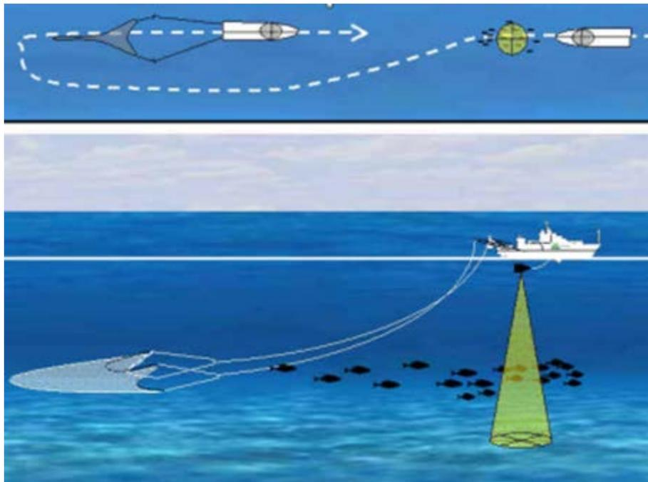
**Figure 5.3** The use of a pelagic, or semi-pelagic, trawl during a hydro acoustic survey. Fish concentrations are encountered during sailing of an acoustic transect. The vessel interrupts the survey, turns and shoot the net to target the fish schools.
