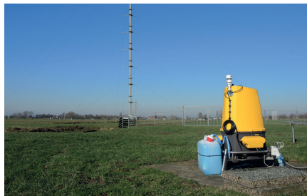
ZephIR 300M wind lidar at CESAR Observatory in Cabauw, the Netherlands
