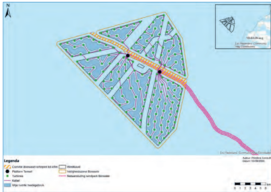
Figure 10-a: The available space for potential multiple use in the Borssele wind energy area (9,800 hectares).
