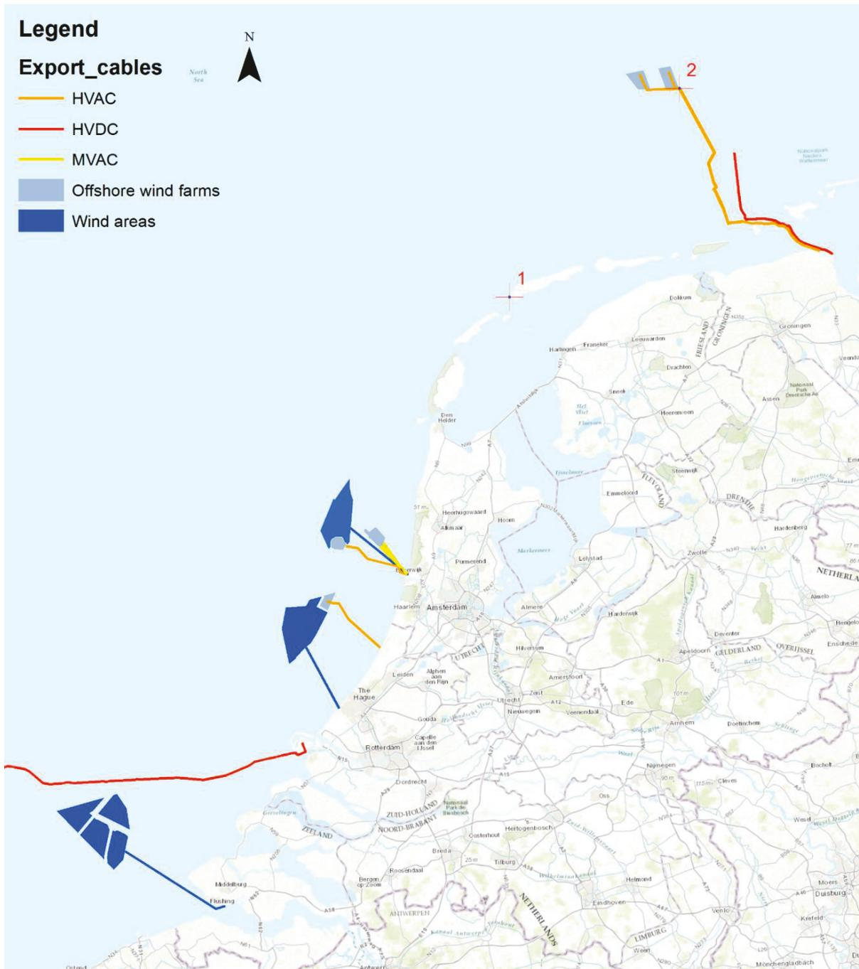
Figure 24: Subsea power cables (red: HVDC, orange: HVAC, yellow: MVAC) and current and planned OWFs (current: light blue, planned: dark blue). Figure is compiled based on currently available information, cable routes of the planned wind farm areas are therefore indicative.
