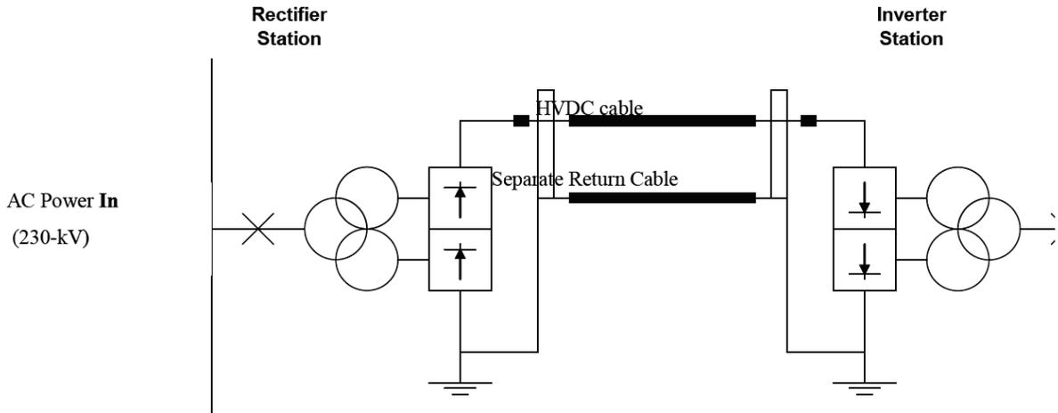
Figure 35: Example of a monopolar DC cable system with a separate return conductor (SRC; Exponent, 2001).
