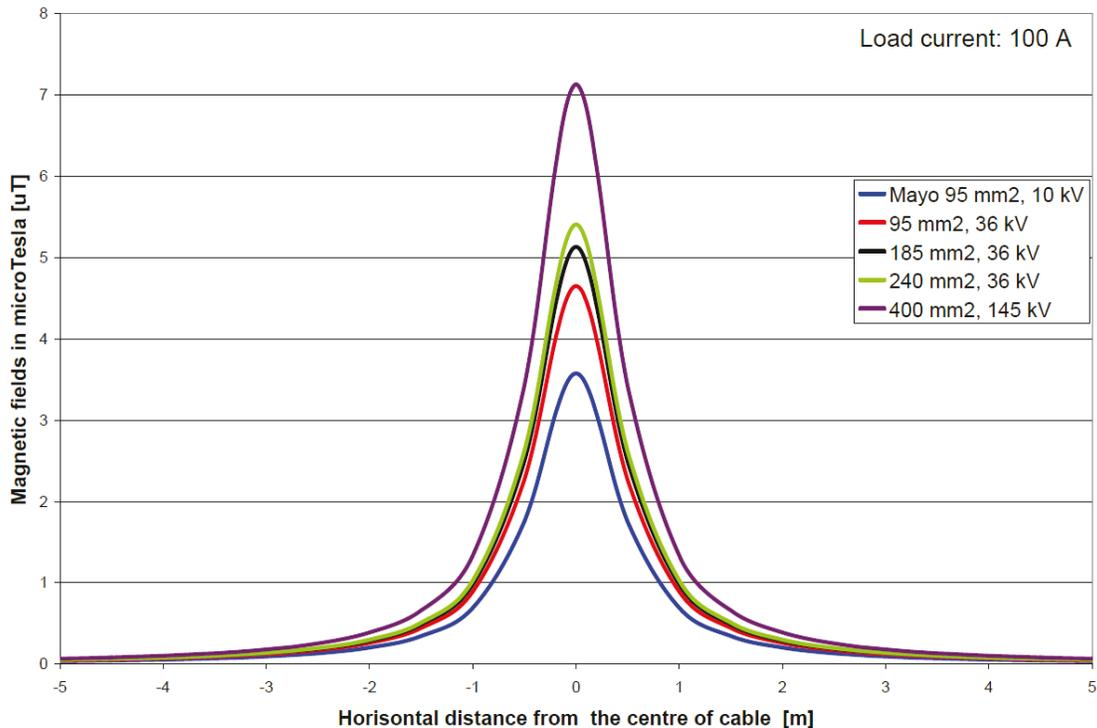
Figure 17: Calculated magnetic field intensities for different types of three phase AC subsea power cables along a line at the sea bottom (Olsson et al., 2010). The cables are buried 0,5 meter under the sea bottom.
