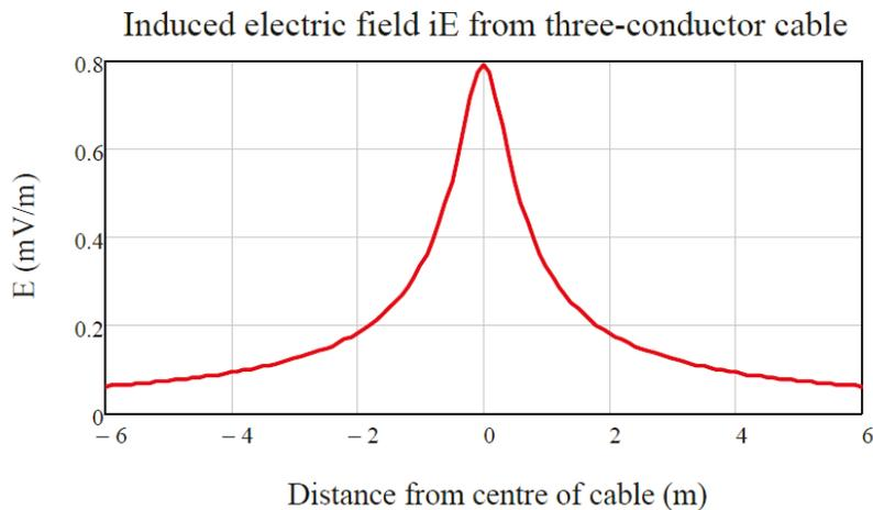
Figure 23: The induced electric field calculated along a profile on the sea bottom perpendicular to a three-conductor AC cable buried 0.5 m assuming a current of 100 A.
