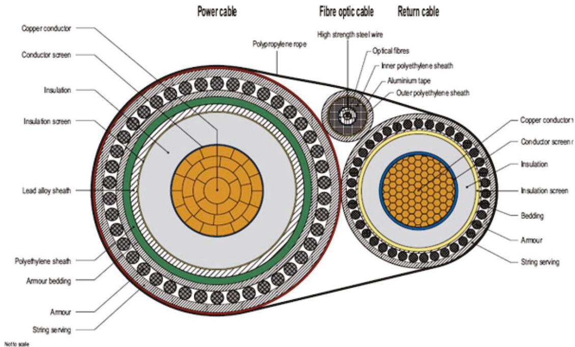
Figure 37 Monopolar DC cable system with a Separate Return Cable (SRC; TPC 2001).
