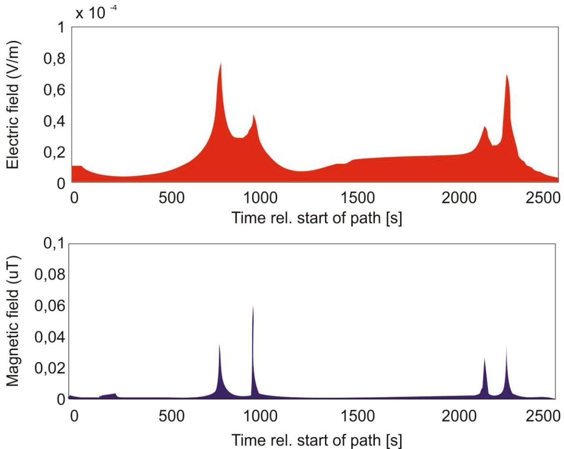
Figure 19: EMF measurements crossing the Northwind and CPower export cables (after Thomsen et al., 2015). The first peak from the left is the Northwind cable and the second the CPower cable. The third is the CPower cable and the fourth the Northwind cable. The upper panel shows the electric field and the lower panel the magnetic field (illustration based on presentation of MARVEN project).
