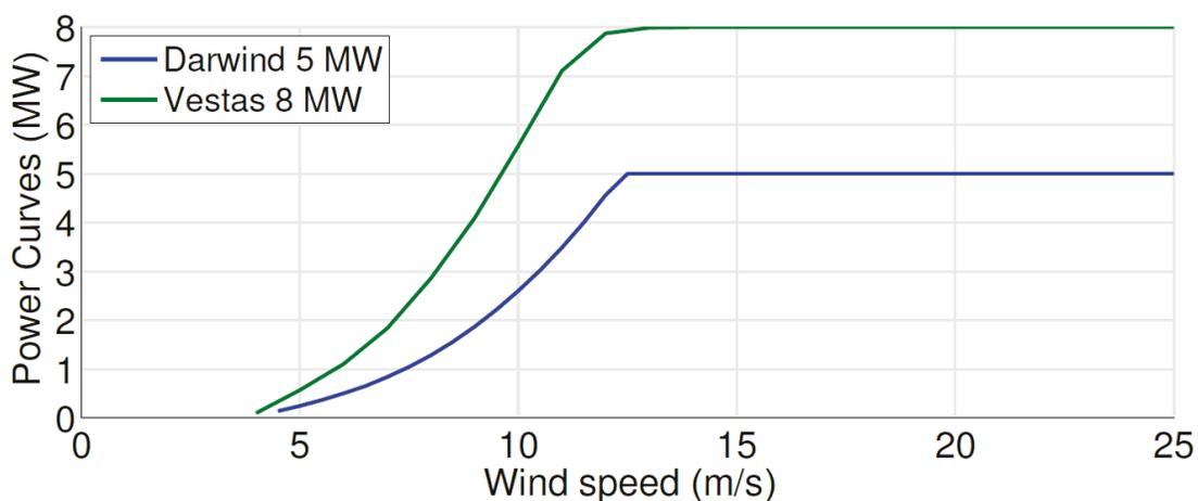
Figure 14: Power curves of two windturbines, showing output power in relation to wind speed (Rodrigues et al., 2015).
