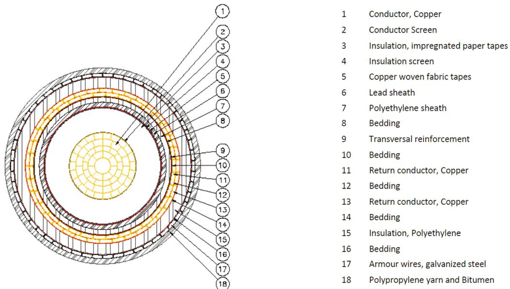
Figure 36: Monopolar DC cable system using coaxial cable with an IRC (Exponent, 2001).
