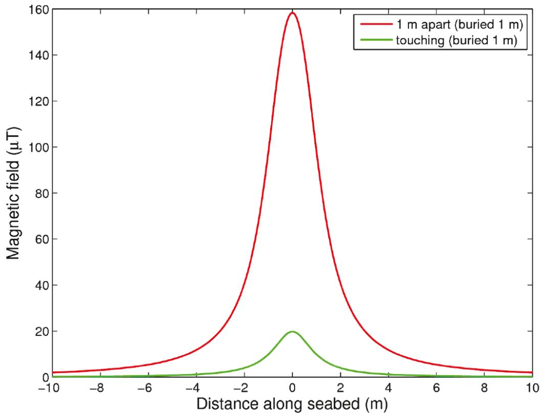
Figure 21: Modelled profile of a DC magnetic field from a subsea 200kV cable operating at 400 MW without taking the geomagnetic field into account (Exponent and Hatch 2009).
