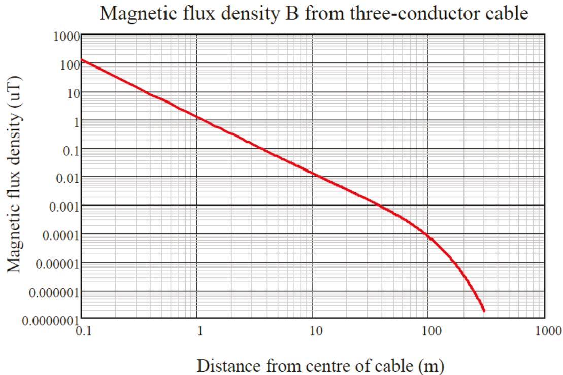
Figure 18: Modelled magnetic flux density in  $\mu\text{T}$  from a three-conductor cable, as a function of the distance from the cable. The current is 100 A, the separation between the conductors is 7 cm and the conductivity of the seawater is assumed to be 3.5 Siemens/m.
