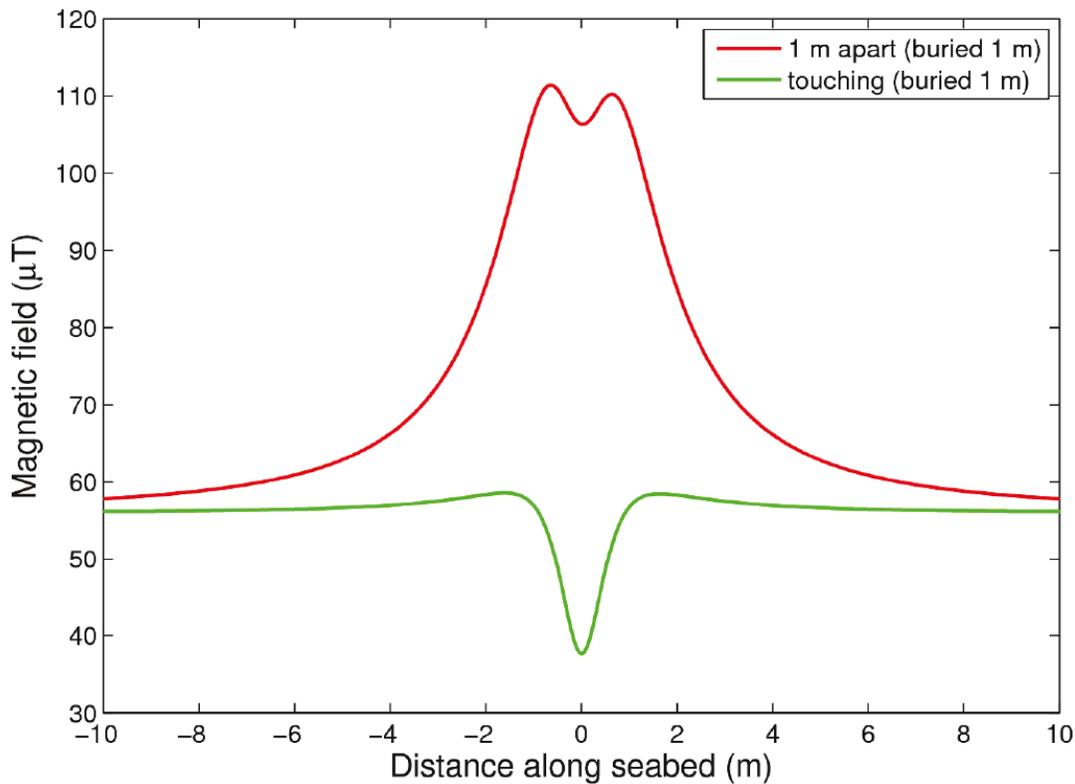
Figure 22: Modelled profile of DC magnetic field from a subsea  $\pm 200$  kV cable operating at 400 MW when orientated NNE and including the geomagnetic field (Exponent and Hatch 2009).
