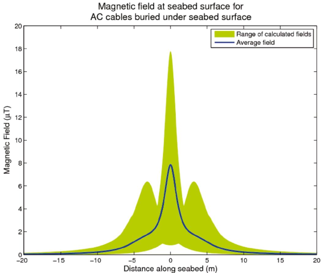
Figure 16: Average modelled magnitudes of electromagnetic field intensity at the seabed for 10 AC cables (Normandeau et al., 2011).
