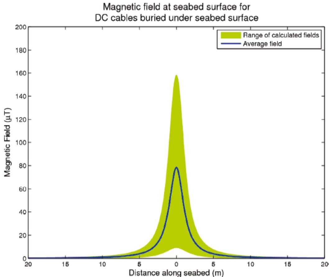
Figure 20: Average modelled magnitudes of electromagnetic field intensity at the seabed for 9 DC cables (Normandeau et al., 2011).
