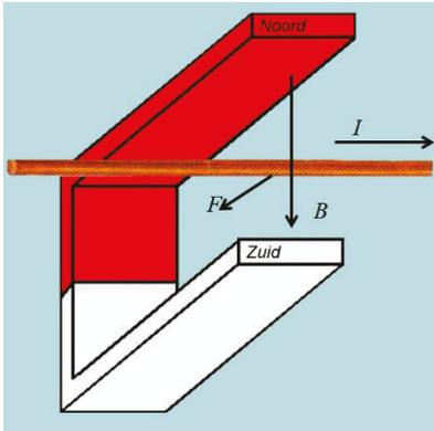
Figure 10: Sketch of the Lorentz force ( $F$ ) in a magnetic field.
