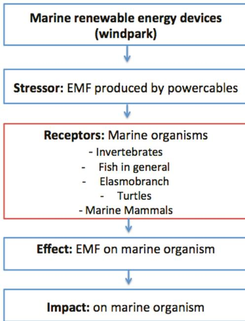
Figure 26 Schematic overview of impact of EMFs on marine life
