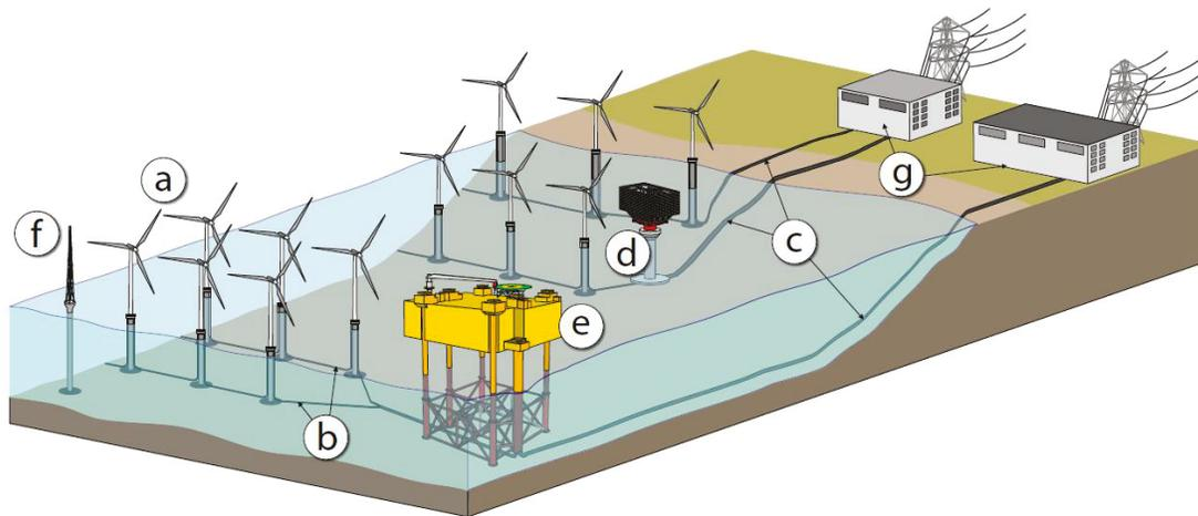
Figure 13: Typical OWF lay-out with the main components of an OWF: (a) Wind turbines; (b) Infield cables; (c) Export cables; (d) Transformer station; (e) Converter station; (f) Meteorological mast; (g) Onshore stations. (figure from Rodrigues, 2016).
