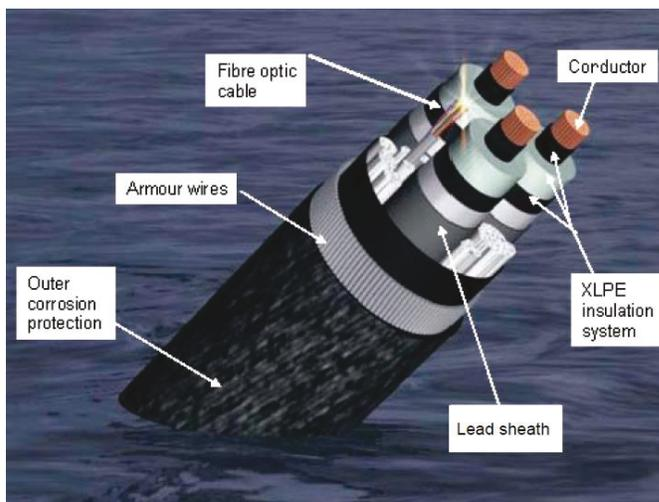
Figure 34: Sketch of a typical subsea high voltage AC cable which displays the three phase conductors and the surrounding sheathing.
