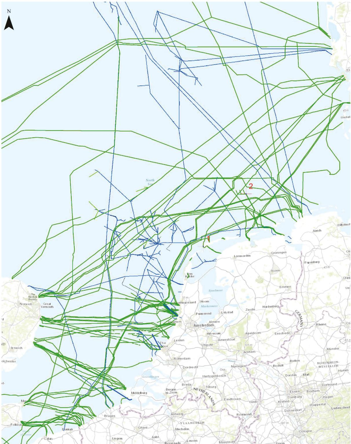
Figure 25: Cables (green) and pipelines (blue) in the North Sea.
