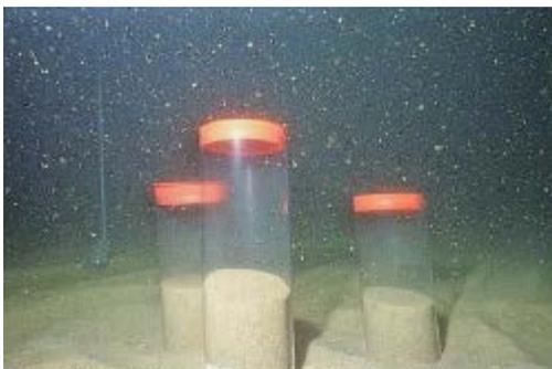
**Figure 5-4.** Sediment core samples, taken from Leonhard & Pedersen, 2006.
