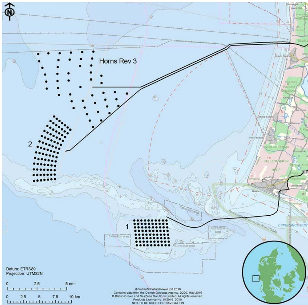
**Figure 5-3.** The locations of the windmills in the wind farms Horns Rev I, II and III (under construction). Taken from: [https://corporate.vattenfall.com/globalassets/corporate/about\\_energy/3c\\_map\\_horns\\_rev\\_123.png](https://corporate.vattenfall.com/globalassets/corporate/about_energy/3c_map_horns_rev_123.png).
