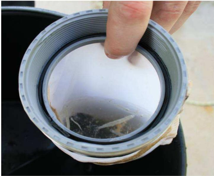
*Figure 3.5. The codend with the plankton sample.*
