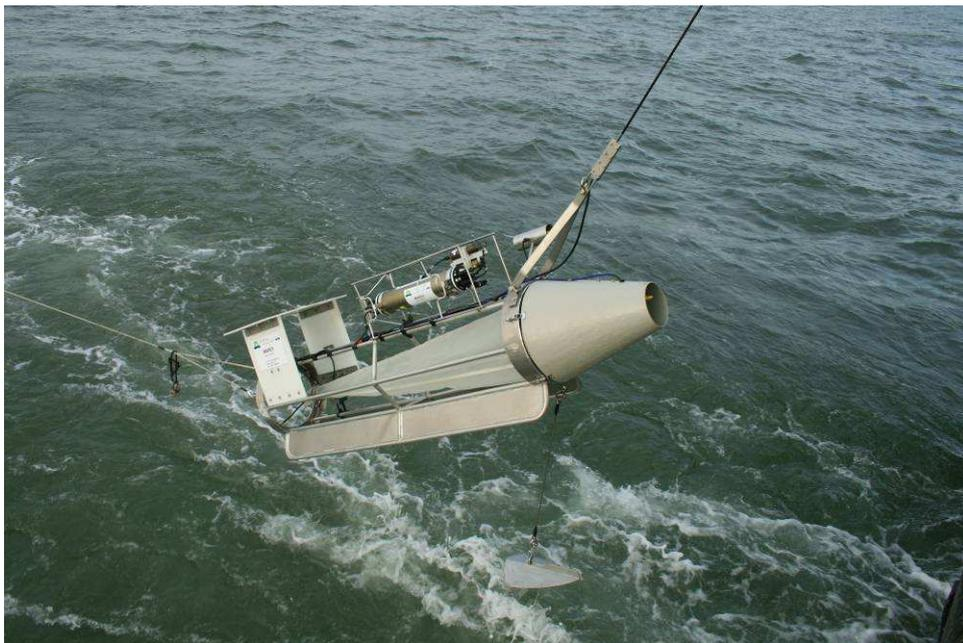
Figure 3.1. Gulf VII plankton sampler.
