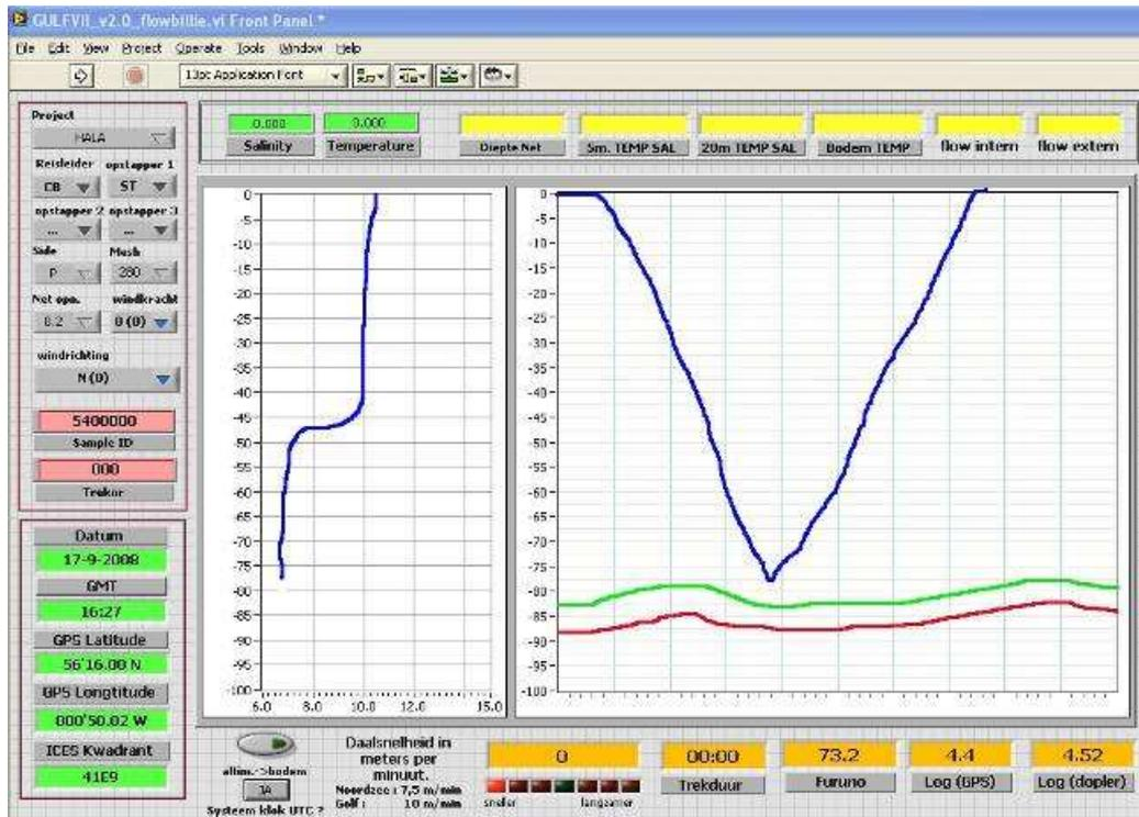
Figure 3.2. Illustration of an oblique haul in the Labview program. In the right frame: The blue line shows the depth profile of the plankton sampler, the red line is the sea bottom depth, the green line is the 5 meter above the bottom safety line. In the left frame: The blue line shows the temperature through the water column.
