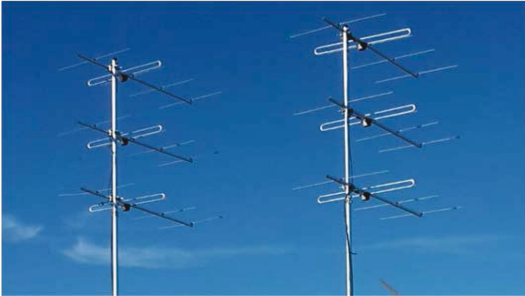
Figure 2.2: The measurement setup for comparing the signal strength for different antennas.
