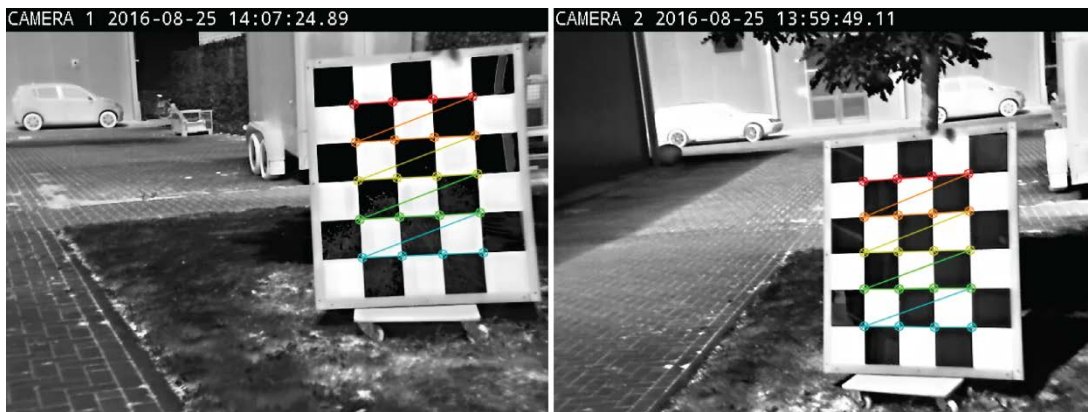
Figure 13: A few examples of the calibration pattern recorded by the long-wave infrared camera. The detection of the chess-board corners are drawn on top of the raw camera image.
