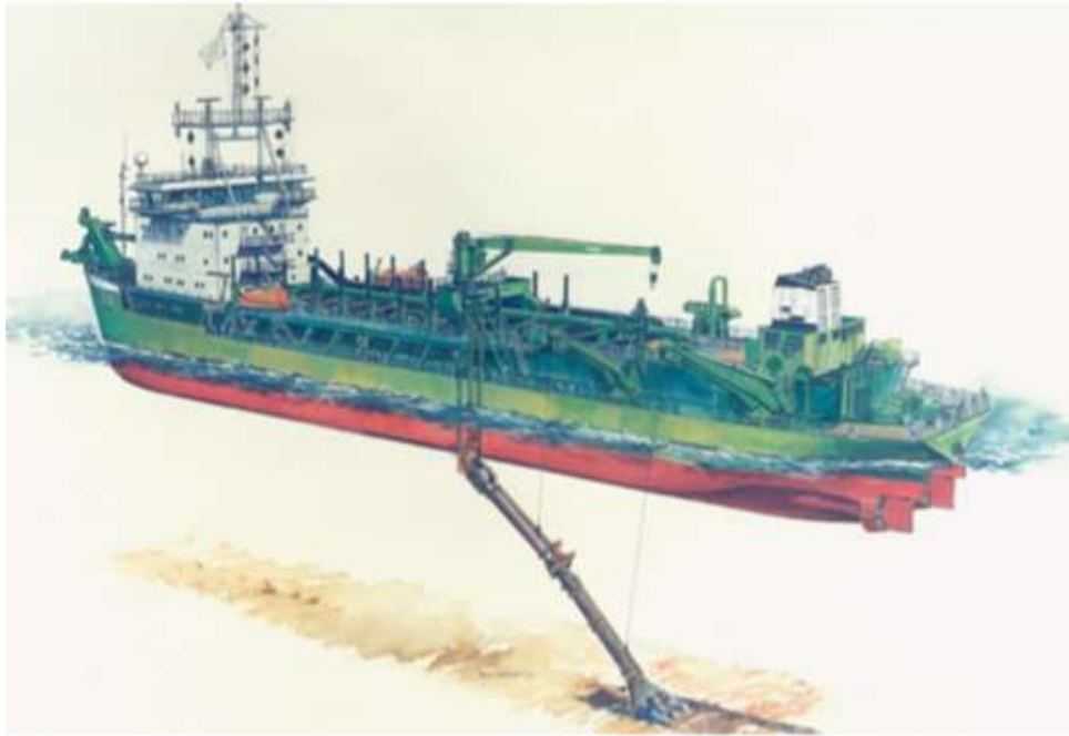
Figure 5. Illustration of a trailing suction hopper dredger. (van Duin et al. 2017)
