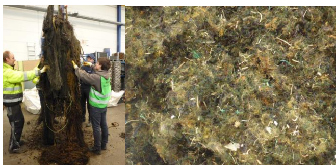
Pre-processing and sorting of retrieved fishing gear (left), cleaned and shredded for further testing (right), images © Andrea Stolte/WWF.
