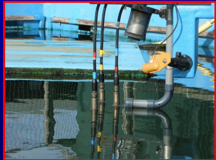
Hydrophones just below water surface, at location of the seals' ears.
