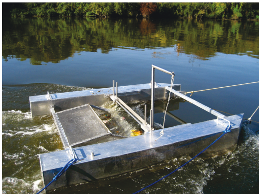
figure 2: Waste Free Waters sampler (Mk-I)
