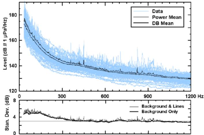
Measured underwater noise source spectra of merchant ships (blue curves) and the ensemble average spectra (black curves: 'Power mean' refers to the energetic average, while 'DB mean' presents the average of the dB-values), with an estimation of the ensemble standard deviation (lower figure), from Wales & Heitmeyer (2002).
