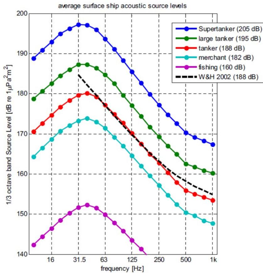
Figure 6: Comparison of source levels from merchant ships (average) (source: Ainslie et al., 2009). W&H 2002 stands for Wales & Heitmeyer (2002), who made an estimation of the ensemble standard deviation.
