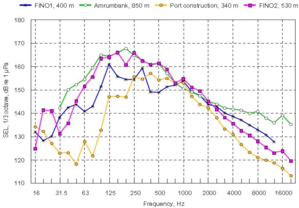
Figure 1: Overview of Third-Octave band spectra of the single stroke SEL of some of the monopile driving operations from different wind farm, data from Nehls et al. (2007) in Ainslie et al. (2009). (Figure from Ainslie et al., 2009).
