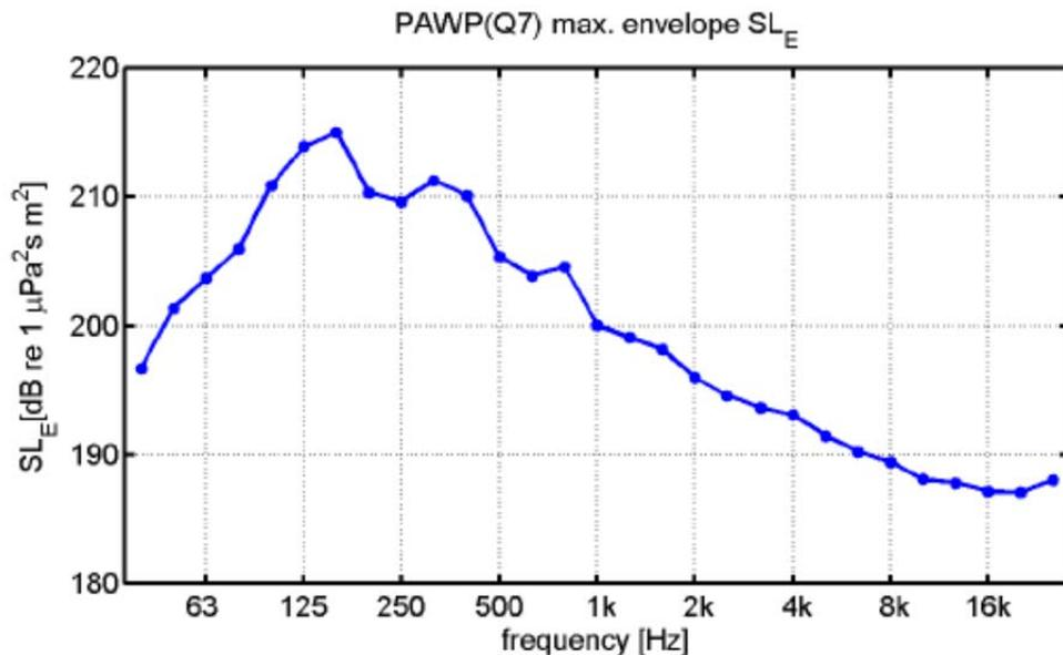
Figure 2: Estimated upper limit of the energy source spectrum (1/3 octave) for underwater noise while pile driving based on measurements during the building of the wind farm Prinses Amalia (Q7). Figure from TNO, 2015.
