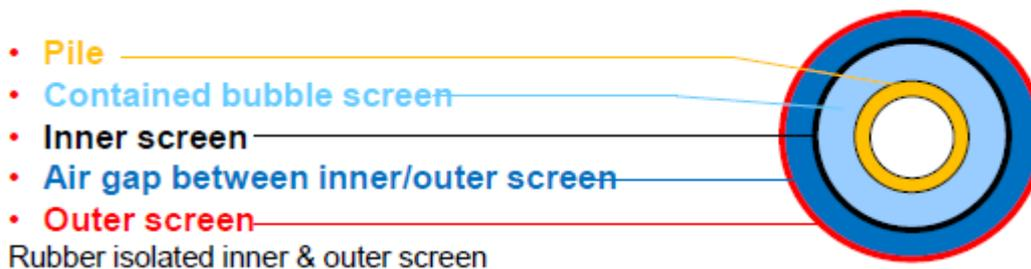
**Figure 14 : Cross section of a noise mitigation system (source IHC Hydrohammer, 2014)**
