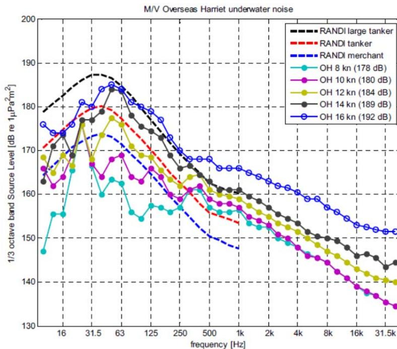
**Figure 7: Relation between the reduction of speed and the production of underwater noise for the overseas Hariette (picture from Ainslie et al., 2009).**
