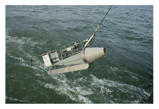
Figure 3.1. Gulf VII plankton sampler.
