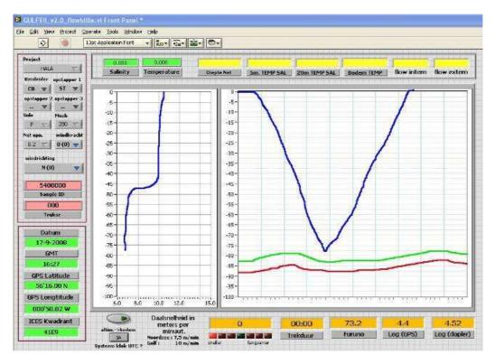
Figure 3.2. Illustration of an oblique haul in the Labview program. In the right frame: The blue line shows the depth profile of the plankton sampler, the red line is the sea bottom depth, the green line is the 5 meter above the bottom safety line. In the left frame: The blue line shows the temperature through the water column.
