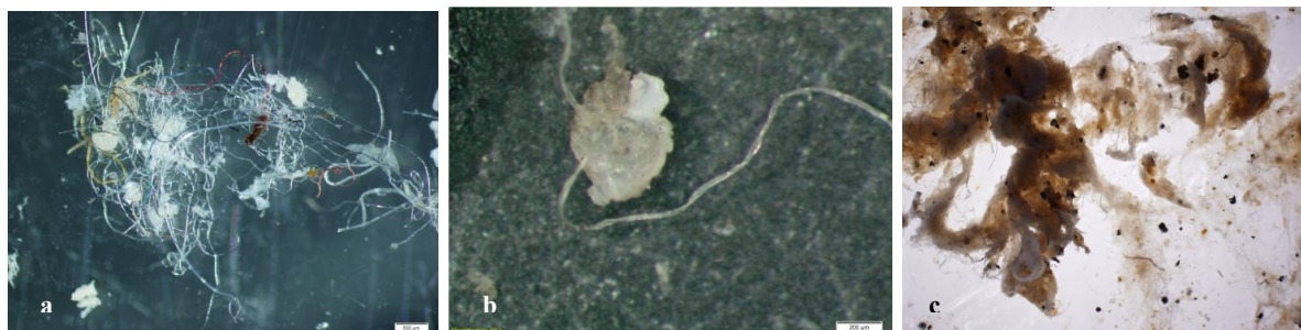
Figure 35. Fibres were regularly observed and they occasionally caused hindrance for microscopic study, such as (a) A clew of polymeric fibres found in the Rhine River (Bad Honnef) holding target MPs. Scale bar = 0.5 mm. (b) A scrub particle and a polymeric fibre molted together. Scale bar = 0.2 mm. Picture taken in pilot phase after \text{HNO}_3 digestion. (c) Lumps of (suggested) cotton fibres found in Meuse river (sample E14, 0.250-
