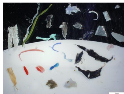
Figure 14. Examples of the group of so called miscellaneous MPs, in the size range 0.250-5 mm observed in Rhine river sample L16. Scale bar = 2 mm
