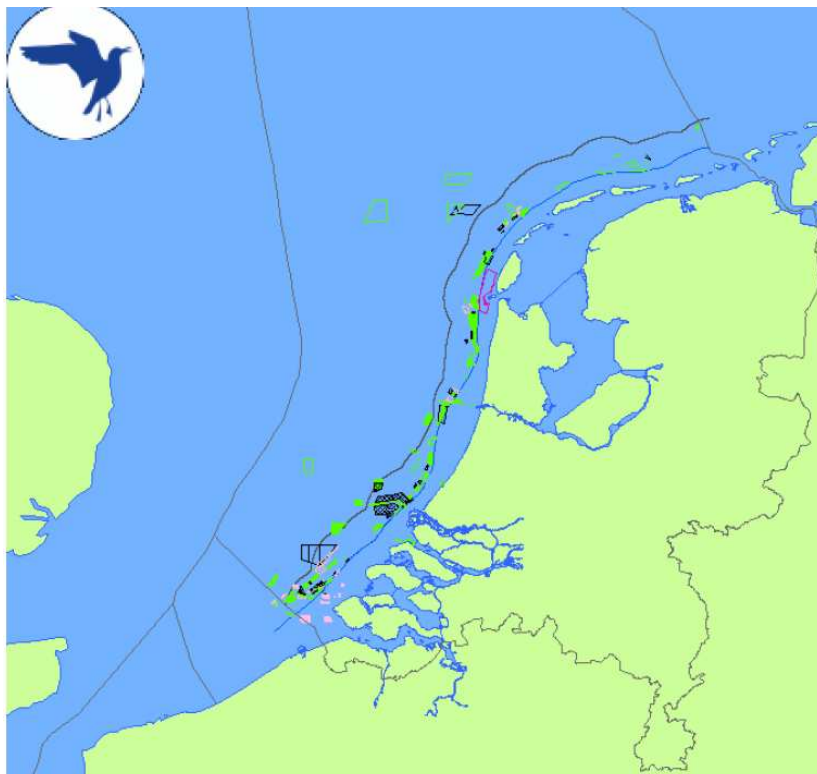
Figure 3.2 Map showing areas used for sand and shell extraction ( www.noordzeeatlas.nl ). Sand extraction is indicated in green, shell in red colors.
