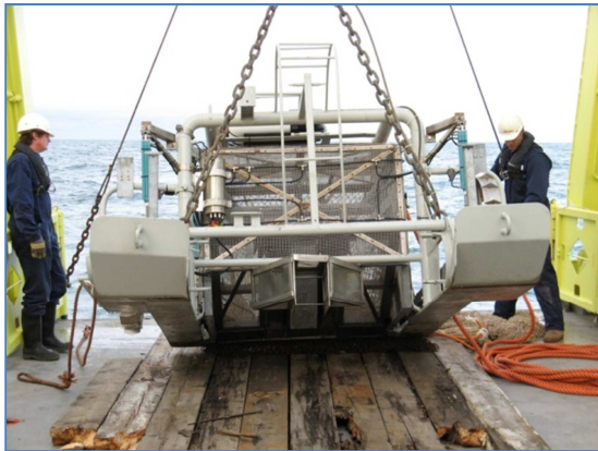
Figure 13. Megabenthos: Deep Digging Dredge (Triple-D: 2008 version: ~ 1500 kg).
