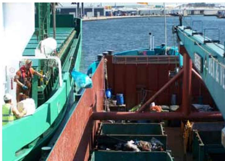
Port reception facilities for taking in shipping waste
